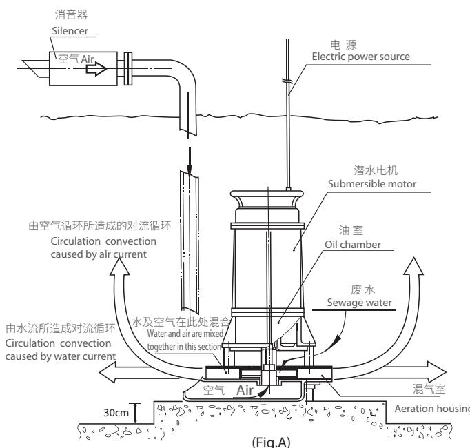
Submersible aerator-AR utilizes the rotation of the impeller coupled directly to the motor to create a centrifugal force, which makes local low pressure suck in water. Meanwhile the entrance of the Impeller results in vacuum to draw air from atmosphere. Water and air mix in the channel of aeration housing. The air-water-mixture current is discharged speedily by the centrifugal force.
